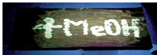
Figure 14. Photograph of an aluminum foil covered by a thin layer of the dry complex cis-6 ( \approx 5 mg on a 12 \times 5 cm surface) exposed to the radiation of a common UV lamp for TLC analysis, at a wavelength of \approx 385 nm. The emission is restricted to areas in which the layer was treated with drops of CH 3 OH.
